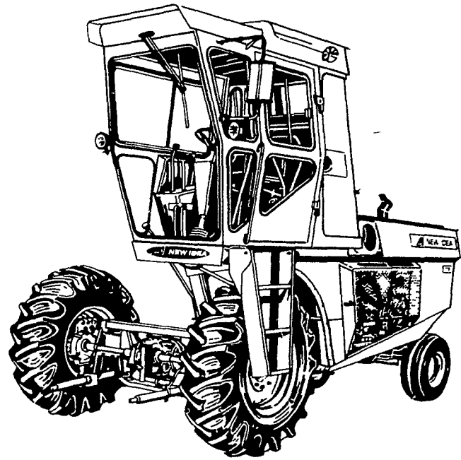
Two hydrostatic Units 138 & 175 brake horsepower turbocharged diesels
