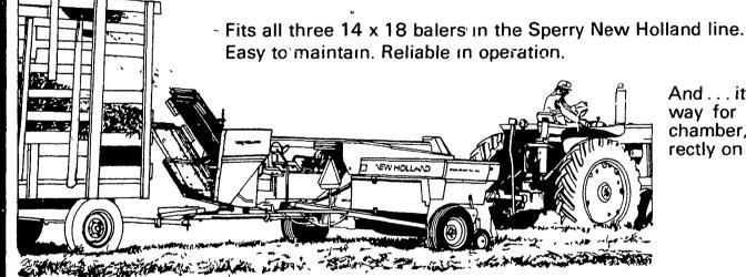
And . . . it swings up, out of the way for easy access to bale chamber, or to drop bales directly on the ground.
