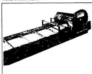
Double #55 Chains with 15" Oak Wood slats Carry Feeding Material in a 20" Wide Conveyor Standard Conveyor length is 16 ft Shorter units are made to accommodate every requirement. Hopper (not shown) for input of feed material is available and will fit on top where needed. Extra slack in conveyor chain can be adjusted at drive end. Bottom Side Conveyor with Chain Return on top available. Incline-to-level Units made to order.
