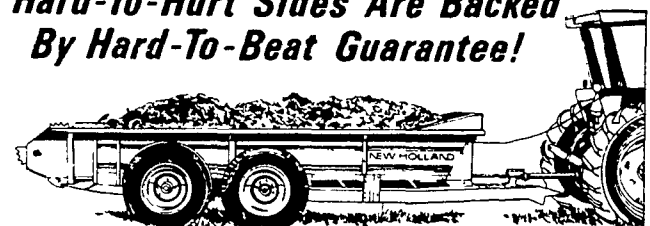
MODEL 791 , with upper beater here, spreads its 419 cu. ft. load in less than two minutes.
