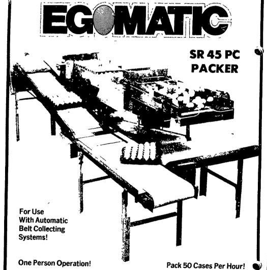
The spring cushion conveyors, for more gentle and positive egg handling, take the eggs thru the disc type orientors, which softly place them, points facing the same direction, into our blue cups. Here the operator merely places the package over the eggs.
