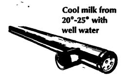
The pre-cooler from Top Line uses well water to cool milk from 20-25 degrees in line before it hits the tank. This in-line pre-cooler can cut compressor time in half, reduce power costs by taking the strain off your condensing unit and relieves the refrigeration load on your bulk tank. Easy to clean in place and easy to install. Sized to fit your system.
