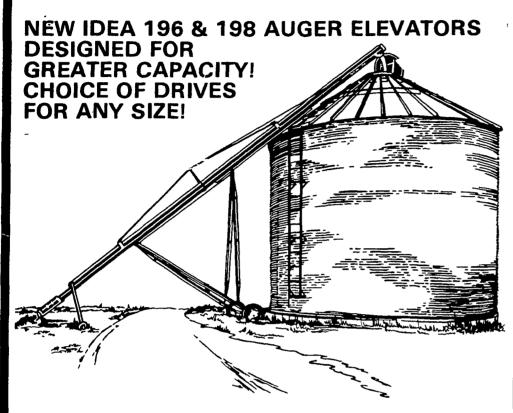
You'll like New Idea's all-purpose auger elevator with the big capacity for high-or-low-moisture corn, milo, oats, wheat, barley, soybeans and other free flowing grain. Choose from 27 to 60 foot lengths. You'll get delivery heights from 17 to 41 feet at a 45 degree operating angle.
