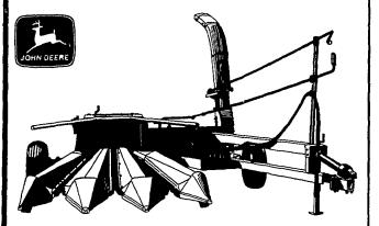
Exclusive J-knife cutterhead works like a paddlewheel, provides greater chopping efficiency These knives, the slip-clutchprotected feed-roll drives, and many other No silo **too tall...** for this 1000-rpm **Forage Blower**
