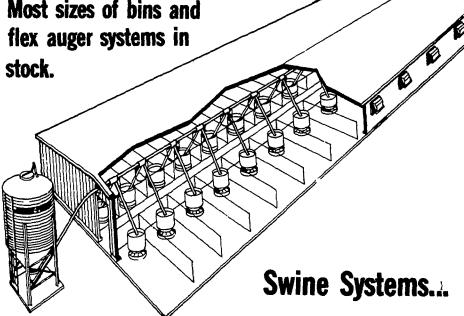
Both rugged and versatile, the Flex-Auger System easily adapts to most hog feeding operations. The Chore-Time centerless auger delivers feed from bulk bin to all feeders located throughout the house. Much of the labor required with other methods is eliminated. The Y outlet drop assembly (illustrated above) or single units can be installed in most any position desired. Feed level is easily controlled by adjusting the height of the drop.
