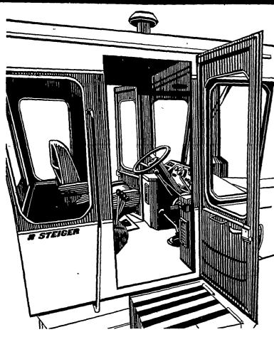
The Steiger cab is rock solid, with two doors allowing entry and exit from either side. Heater and air conditioner are standard, so is AM/FM radio and stereo tape deck. The comfortable and quiet environment inside the slightly pressurized Steiger cab helps ensure that when you climb down at the end of the day, you will be less tired and more relaxed.
