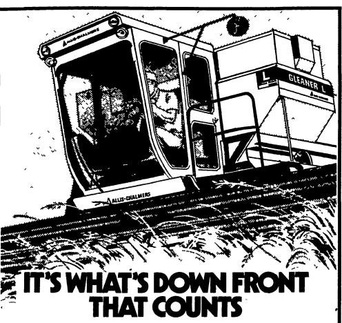
Come in now! Let us show you how the down-front cylinder in Allis-Chalmers *Gleaner* combines gives you complete crop control (only 15½ inches from back of header to cylinder) You get maximum threshing over the full 8-bar cylinder, so you can harvest bigger crops cleanly, quickly even under tough combining conditions.
