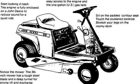
Put it in gear. The shifton-the-go transmission offers a neutral start for safety . A reverse gear And 5 forward speeds-14 to 53 mph on the 66, 1 5 to 5 7 mph on the 68
