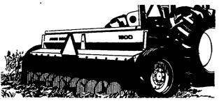
Interseeding pastures is easy with exclusive PTO-driven cutter wheels that rotate in the direction of travel to open narrow miniseedbeds through hard soil, sod, and stubble Seed is deposited into the trenches and then tamped in by narrow firming wheels. Grass or grain models are available
