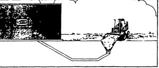
Manure is scraped or drained to a ground-level hopper pumped underground and up through the bottom of your Sealstor Manure Control Center
