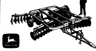
Here's an ideal disk for primary tillage Weight of 123 to 159 pounds per blade lets you cut deep and fast Choose working widths from 111/2 to nearly 15 feet
