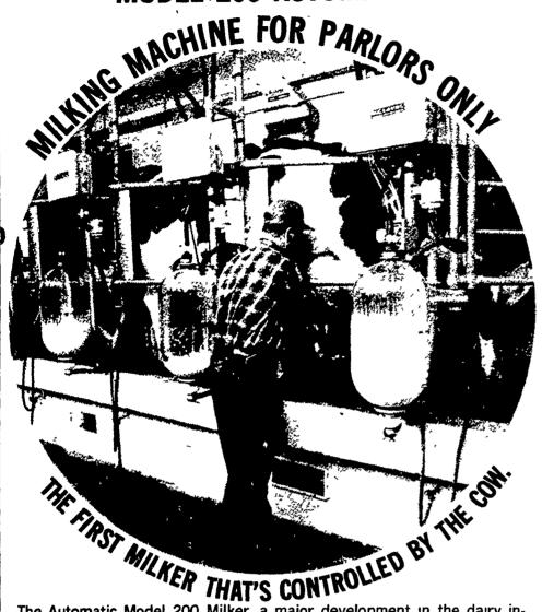
The Automatic Model 200 Milker, a major development in the dairy industry, is the first milker that is controlled by the cow. When the cow is ready, the machine begins to milk and an indicator light goes on to tell the operator that it is milking. The Model 200 automatically stops milking when the cow is through. The indicator light will then go out telling the operator that the cow is milked out.
