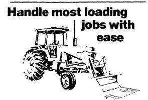
We ve got the John Deere 148 Loader on the lot-ready for your inspection. Put this loader on your medium-size John Deere Tractor\* Lift 11/2 tons to 101/2 feet Break out 4 700 pounds
