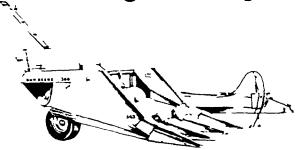
Through the first elevator, & 2400-cubic-footper-minute air blast removes stalks and trash Stalk ejector rolls remove ears and eject stalks Above the husking bed a 3400-cfm blast loosens husks effectively Aggressive husking rolls complete the cleaning job
