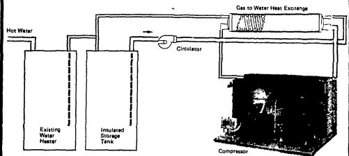
Make your own free Hot water from your existing refrigeration compressor on bulk tank, cooling rooms, freezers, and air-conditioners, etc. Also
