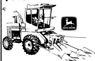
John Deere Self-Propelled 5200 and 5400 Forage Harvesters are not just pull-type units with engines added They re SP-built with 9-knife, 24-inch-diameter cutterheads Exclusive J-knives can be held more rigidly Recutter screens have a larger surface area Feed rolls are slip-clutch protected. The power units are loaded with features too. We have one of these giant SP forage harvesters ready for you right now Come by soon and check it out in person
