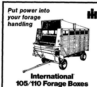
These big boxes hold up to 6 tons of silage to keep you on the move in the field, then unload fast at the front end once you get to the silo. Both models are similar in design The 105 has a 3-speed ratchet apron drive, the 110, a 2-speed roller chain drive
