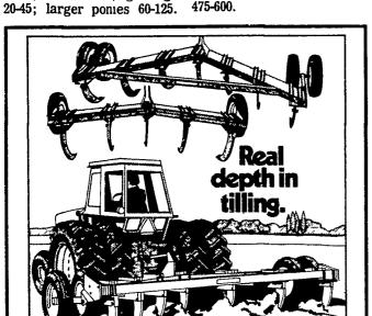
New V-chisel from Allis Chalmers brings you deep down tilling in hardpan condi tions Choose from 5 shank or 7 shank units with single gauge or dual gauge wheels to reguance virtually ends trash build up And shanks feature slip-on points for fast low-cost maintenance and replacement Come in Let us show you
