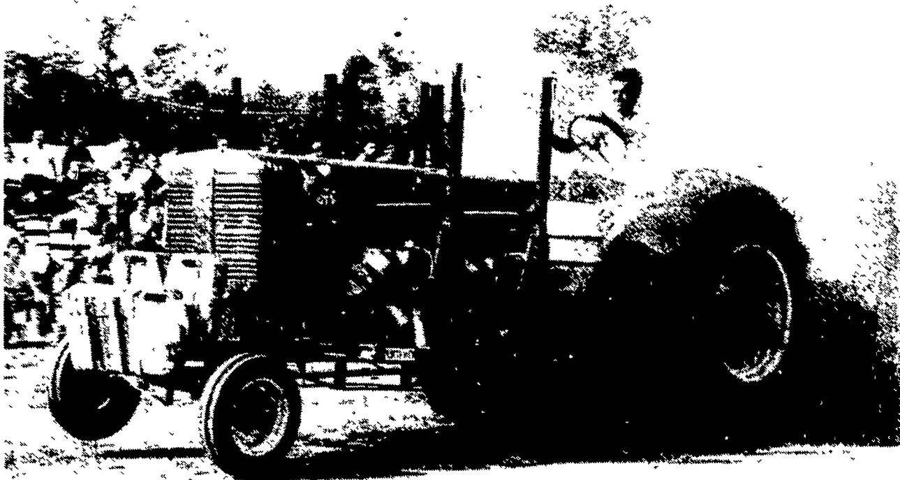
The Bosse Brothers' machine, an IH W9 with four 460 Lincoln engines driven by Carl Bosse of Ada, Ohio.
