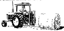
Attach this low-cost big round bale forklift to your tractors 3-point hitch (Category 2) or Quik-Coupler™ hitch and you can lift 1,500pound bales for transport or for loading onto truck beds or trailers
