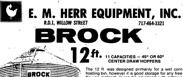
holding bin, however it is good storage for any free flowing material. It can be equipped with either a 45° hopper or a 60° hopper depending on the requirements of the material to be handled There are 6 capacities in the 45° model ranging from 21.5 to 55 0 tons The 5, 60° center draw models have a
