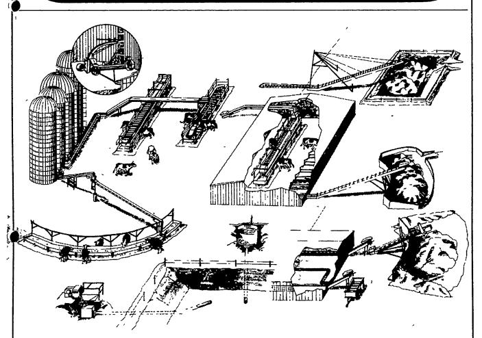
Patz 98B silo unloader 150 cattle feeder 400 cattle feeder 162A circular feeder 101 Taper-Pan Feeder
