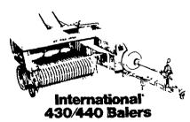
430 - Bales up to 17 tons per hour, twine or wire-tie; 65-in. pickup 440 - Bales up to 19 tons per hour; twine or wire-be; 65-in pickup
