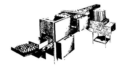
The Staalkat Farmpacker is designed for automatic packing of eggs direct from cages to flats. The Farmpacker has a 50 case per hour capacity and is easily controlled by one operator.
