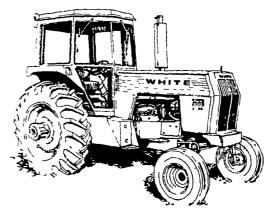
Investment Credit can help you buy this 105 PTO hp<sup>•</sup> White<sup>§</sup> 2-105 Field Boss<sup>™</sup> The 2-105 features a closed center hydraulic system, 3-point hitch, and the 18-speed Over/Under Hydraul-Shift transmission that provides 3-speed snift-on-the go
