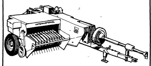
Forget about costly down time and missed bales with the International® All-Twine Balers with the knotter that ties a unique bow-type, double diameter knot that test up to 17 percent stronger than ordinary single diameter knots and does it with all types and diameters of baler twine, without adjustment
