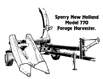
The Sperry New Holland exclusive 12-knife cutterhead is coupled with a P.T.O. driven power sharpener to keep knives razor sharp
