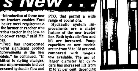
on the model. New filtering and cooling help provide improved hydraulic system durability and protection. All units use a spin-on, micronic, full-flow filter placed in the suction line to remove impurities before they enter the pump, compared with previous model suction line screens and-or return line filters.
