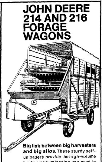
hauling and unloading you need to keep up with modern choppers. The 16-foot 216 with side extensions has a whopping 657-cubic-foot capacity; the 14-foot 214, 574. Five-speed PTO unloading lets you match the discharge rate to blower capacity. Keep your silo filling on schedule with John Deere Forage Wagons.
