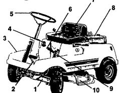
1 Tough automotivetype steel frame 2 Easy stop-and-go pedal driving 3 Rustproof molded fiberglass body 4 Fast, dependable starts
