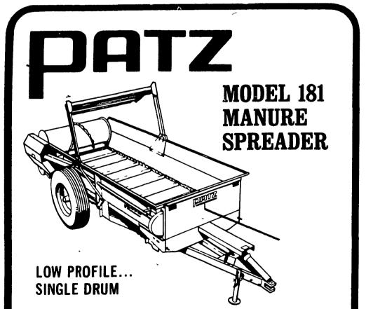
Fits all standard tractor P.T.O.'s ... rugged Patz Model .150 hook-and-eye apron chain ... full 180 bu. capacity ... optional hydraulic end gate retains all liquids within spreader box during travel.
