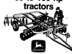
Chop light trash, incorporate chemicals, or make seedbeds with weight-per-blade of 55 to 75 pounds. Cutting widths range from 11 feet 4 inches to 14 feet 3 inches with 714- or 9-inch blade spacing.
