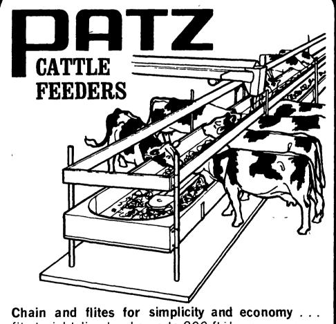
fit straight line bunks up to 200 ft. long . . . move all types of feed smoothly around bunk without sifting or separating.
