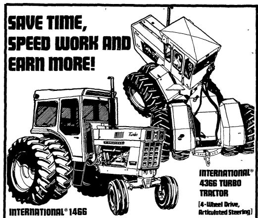
The best tractor for big tough jobs. Its powerful International 436 cu. in. turbo diesel develops 145.7 PTO hp. 8 speeds forward, 4 reverse. Or 16 and 8 with optional shift-on-the-go Torque Amplifier. Smooth hydrostatic steering.
