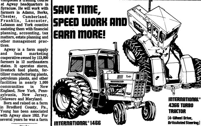
The best tractor for big tough jobs. Its powerful International 436 cu. in. turbo diesel develops 145.7 PTO hp. 8 speeds forward, 4 reverse. Or 16 and 8 with optional shift-on-the-go Torque Amplifier. Smooth hydrostatic steering.
