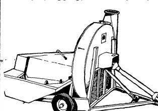
The International® 56 Blower handles 100blows it up to tons of corn silage an hour 100-ft or more
