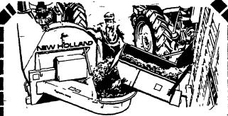
The exclusive whirling table on Models 25 and 27 give the material a "running start" into the blower fan. This means less drag on the fan. more efficient use of horsepower and high capacity. We have these blowers in stock now . . . in a size to fit your needs. Drop in soon to see Models 25 and 27.
