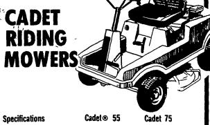
Engine 5 hp 4-cycle gasoline. 1st gear, 2 2 mph, 2nd, 3.3; 3rd, 4 9, Speeds Reverse, 3.3 32" **Cutting** width  $1^{1}/2$ " to 4" in  $^{1}/2$ " increments. **Cutting height** 35" 35" Wheelbase 56" 56" Overall length Inside turning radius 25"
