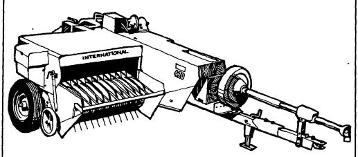
All-Twine Balers . . . with the knotter that ties a unique bow-type, double diameter knot that test up to 17 percent stronger than ordinary single diameter knots .. and does it with all types and diameters of baler twine, without adjustment.
