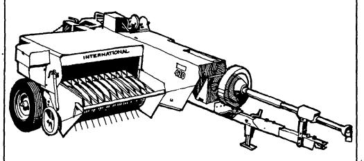
with the knotter that ties a unique bow-type, double All-Twine Balers diameter knot that test up to 17 percent stronger than ordinary single diand does it with all types and diameters of baler twine, withameter knots out adjustment
