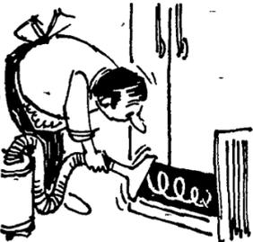
★ Vacuum clean refrigerator coils making sure compressor motor is dirt- and dust-free. Some coils are exposed on the back of the units — access to others is through a removable panel on the front at floor level. Clean at least once each year.
