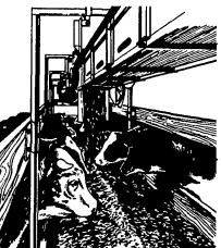
Model 166 Feeders are available for bunks from 50 to 200 feet long, are powered by a 1½ or 2 HP instant reverse motor.
