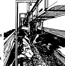
Model 166 Feeders are available for bunks from 50 to 200 feet long, are powered by a 1½ or 2 HP instant reverse motor.
