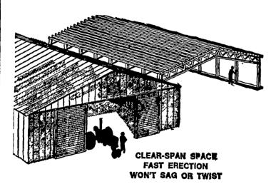
All the brute strength of curved steel is utilized throughout the exclusive framing system of Behlen's new "Tubeline" building. It's designed for strength, and for easy construction. Simple bolt-together connections speed erection. Clear-span design eliminates centerpole installation.
