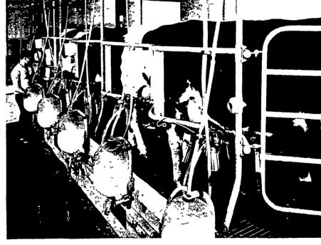
Shown above is a two-man, double-6 herringbone parlor equipped with calibrated, glass weigh jars. This system is ideal for the dairyman who desires to check the production of every cow at every milking. Washes-in-place. The large vacuum reserve near the udder helps to stabilize vacuum at teat.
