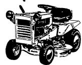
Non-scalp mower trims 1 2 acres per hour at a pass Power take-off points in three locations feed engine power directly to ten attachments that go on and off in seconds
